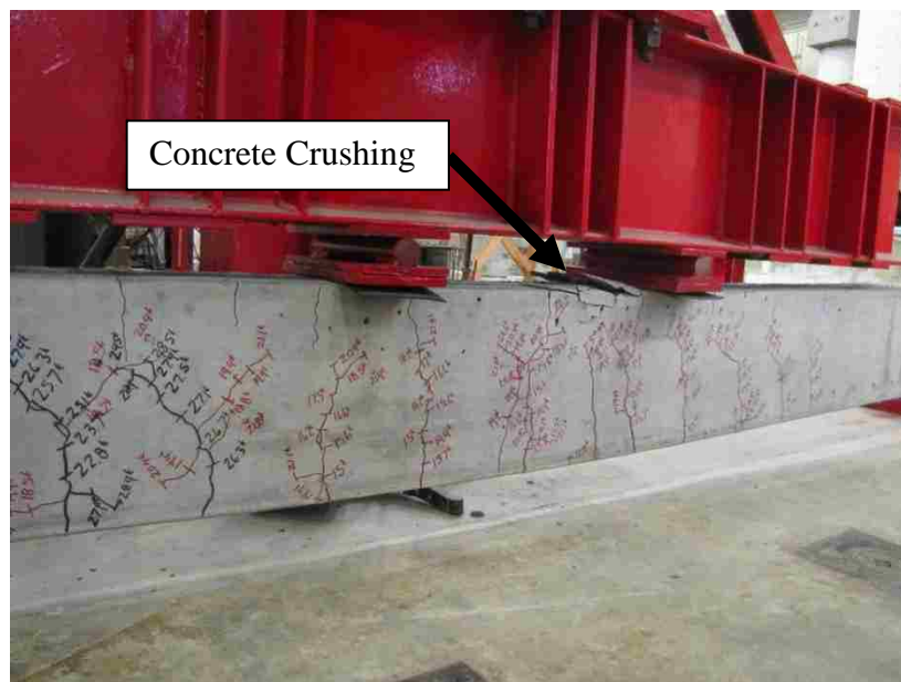
Figure F.31 – S10-2-2_73 at Failure
