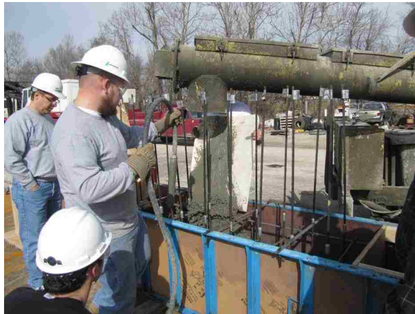
Figure 3.23 – Casting the LBPT Specimen
