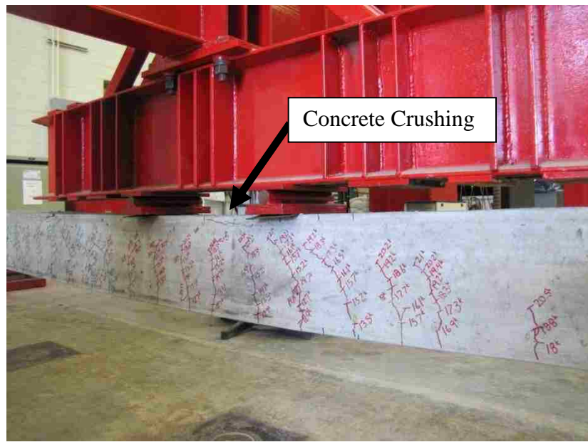
Figure F.7 – C6-2-2_73 at Failure
