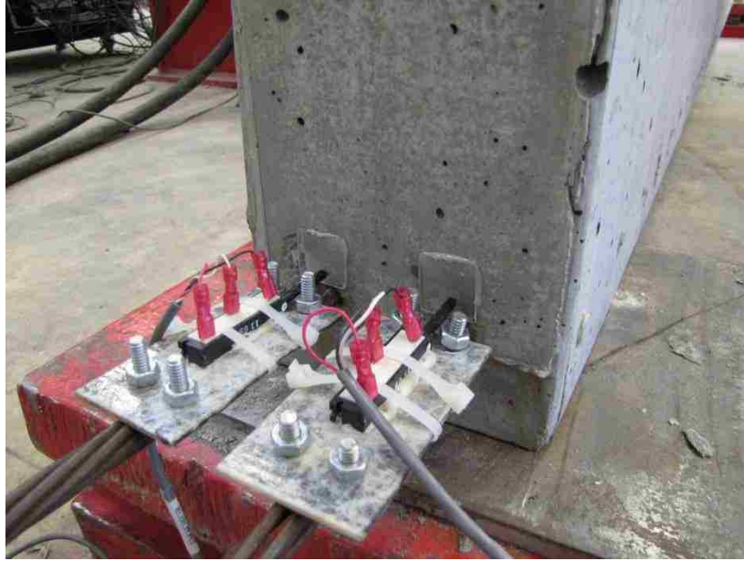
Figure 4.28 – Linear Potentiometer Setup on Four-Point Loading Tests
