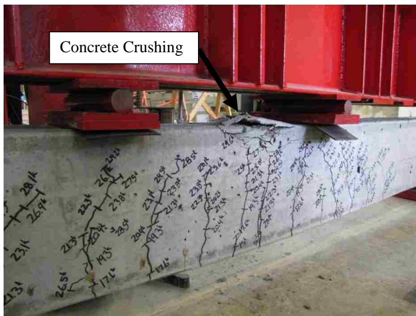
Figure F.21 – C10-2-2_58 at Failure
