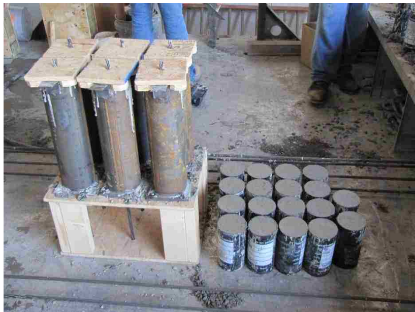
Figure 3.12 – Capped NASP in Concrete Specimens and Cylinders
