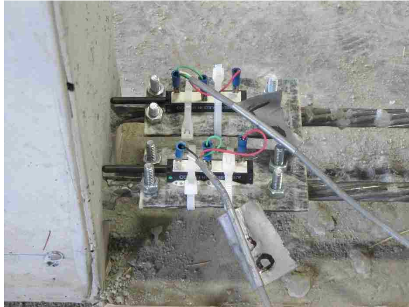
Figure 4.21 – Improved Potentiometer-FRP Assemblies with Zip Ties and Plastic Epoxy (Top) and Gorilla Glue Expanding Foam (Bottom)
