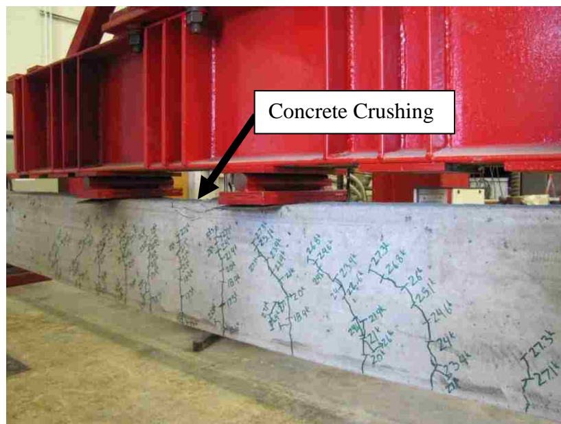
Figure F.5 – C6-2-2_58 at Failure
