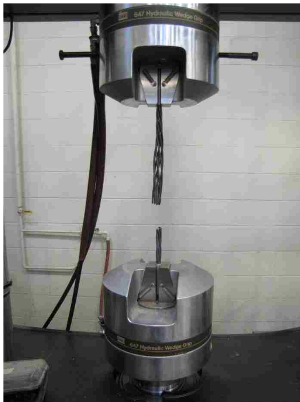
Figure 3.4 – Fractured Tension Test Specimen
