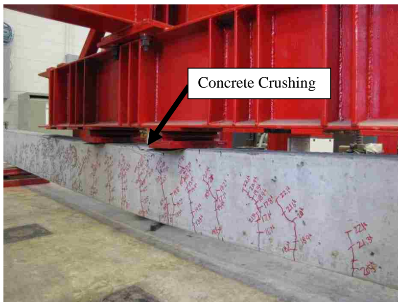
Figure F.19 – C10-2-1_73 at Failure
