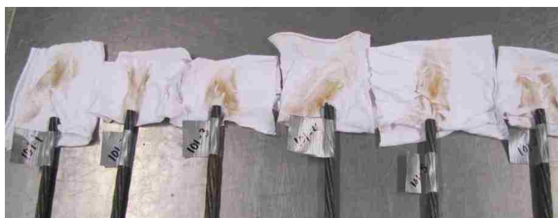
Figure 3.29 – Towel Wipe Results for Strand Type 101
