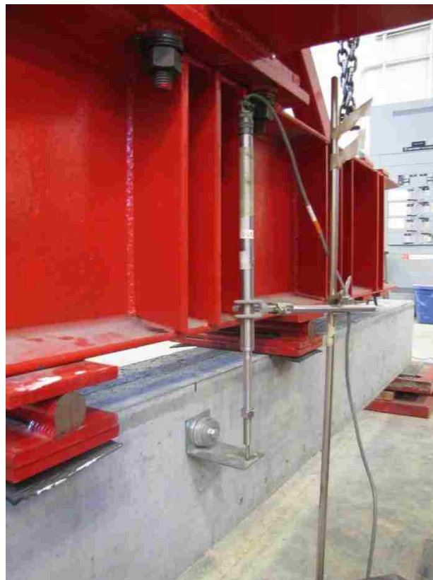
Figure 4.27 – LVDT Setup for Measuring Deflection at Midspan
