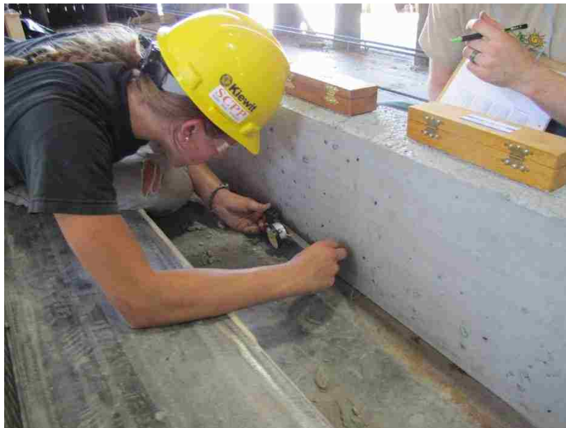
Figure 4.13 – Taking DEMEC Readings
