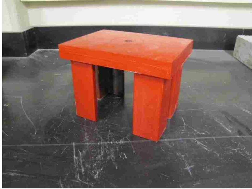
Figure 3.26 – Steel Table for LBPT
