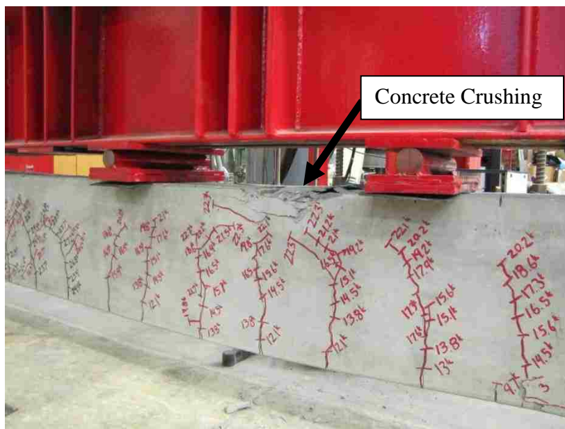
Figure F.11 – S6-2-1_73 at Failure
