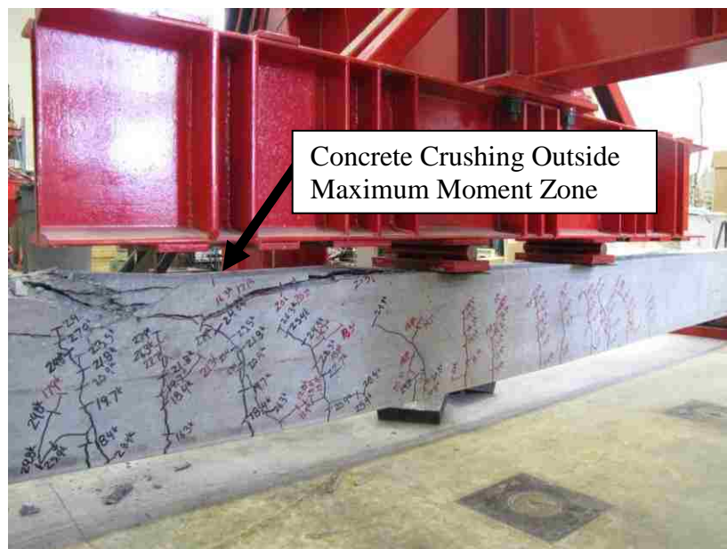
Figure F.15 – S6-2-2_73 at Failure
