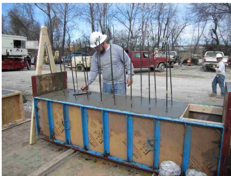
Figure 3.24 – Finished LBPT Specimen
