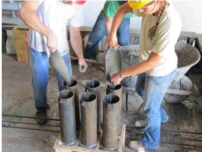
Figure 3.11 – Filling Specimens for NASP Test in Concrete
