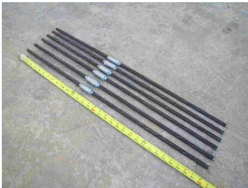
Figure 3.6 – Strands with Bond Breakers
