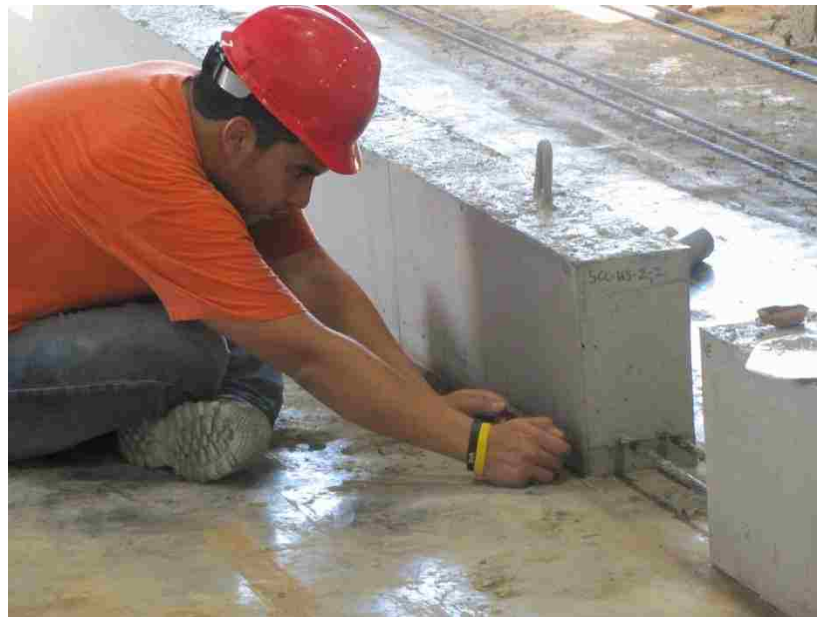
Figure 4.11 – Setting DEMEC Points with Setting Bar
